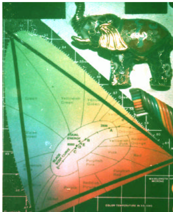
Figure 4. Hologram of the CIE test object recorded with 476, 532, and 647 nm laser wavelengths
